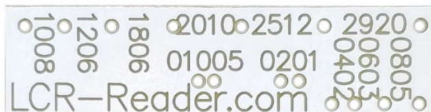
Figure 3. Capacitance offset calibration board.
