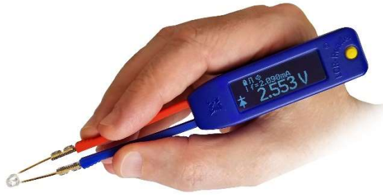
Figure 4. LCR-Reader-MPA testing LED
