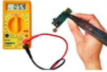
Hand using LED Test Tweezers
