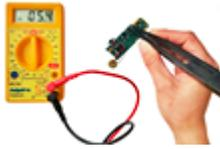
SMD Multimeter Test Tweezers
